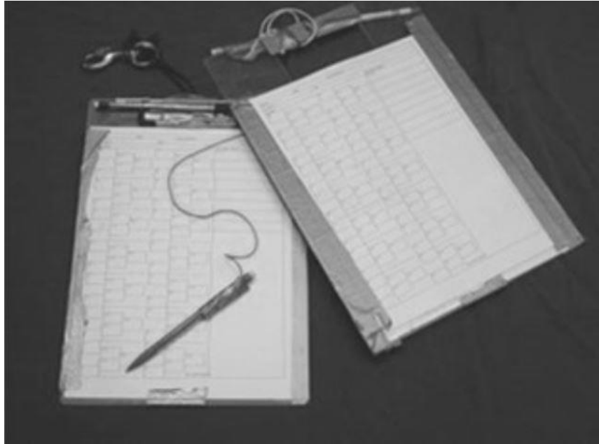
Figure 39. Photograph from the MAST Basic Workshop of the mylar worksheets taped to a clipboard with a pencil so the measurements can be recorded underwater. The clipboards were attached to lanyards to avoid being lost underwater [Source: MAST]
