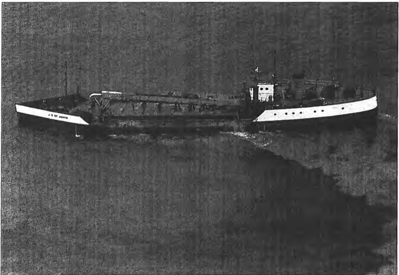
Figure 20. Sand dredge J. S. ST. JOHN working on the Long Point-Erie Ridge (courtesy of Erie Sand Steamship Company). Note turbidity plume at the stern of the vessel caused by fine-grained material washed from the sand.
