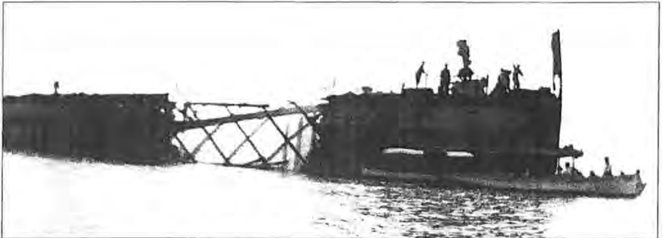
Figure 15. Photograph of the F. H. PRINCE after the second fire on August 14, 1911 which caused the total loss of the vessel (Gordon Wendt Collection). Note the metal reinforcement strapping that was exposed once the wood hull had burned away.
