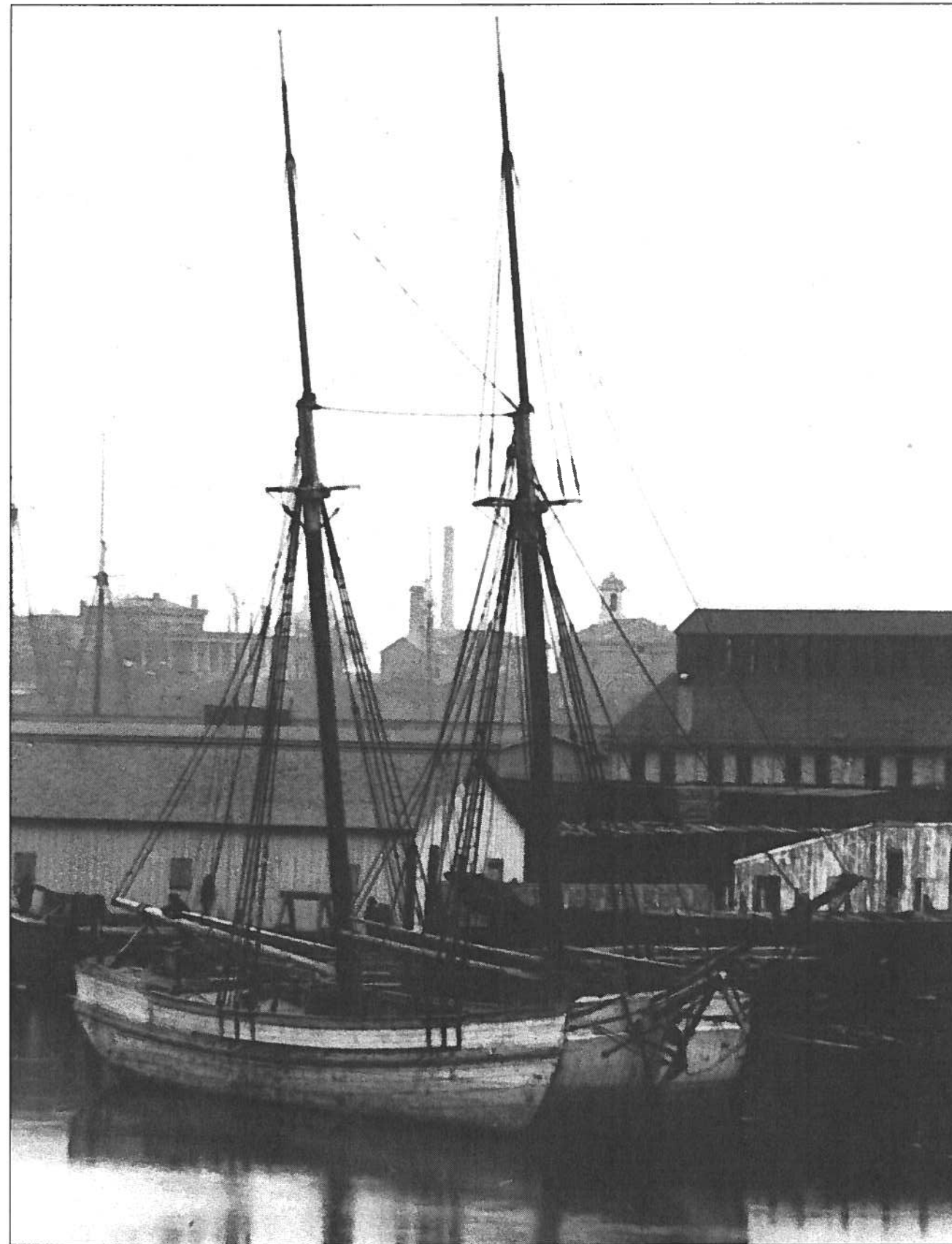
Scow schooner MERCER at Sheboygan, Wisconsin, circa 1890 (Rev. Edward J. Dowling Collection, University of Detroit-Mercy). Built at Erie, Pennsylvania in 1849, 85 x 22 feet; note "spoonbill" bow.
